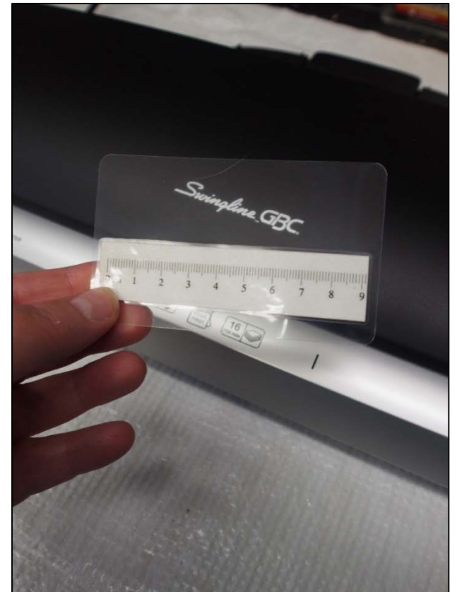
Homemade weatherproof business card-sized ruler made in lamination machine. © Lena Struwe, 2017.
